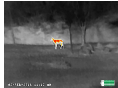
InstAlert: The hottest object in the image is colored while everything else is greyscale
